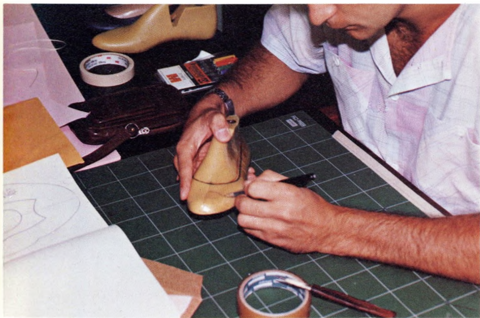
Students at the LIRI training centre in Durban learn to cut patterns for footwear manufacture
