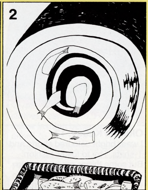
Then the fish are moved into a large cylinder with metal wire inside. The wire turns around, rubbing the scales off the fish as it turns.
