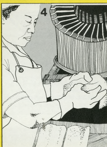
4 The filleting machine is next along the line. It cuts the flesh off the bones. Then the filleted fish is skinned.
