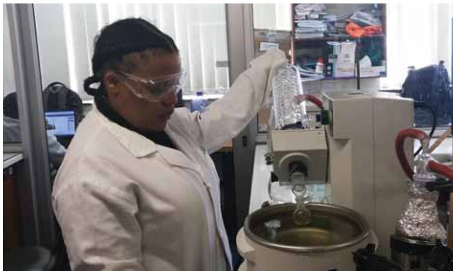
Masego Kotane (MSc) is using the Rotary Evaporator to evaporate solvents for her research project.
