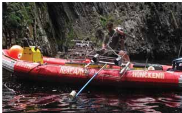
Multiple stereo-BRUV systems can be deployed simultaneously to maximise sampling efficiency. Here, Denham Parker gets ready to deploy the next stereo-BRUV off the research vessel Honckenii in the Tsitsikamma National Park Marine Protected Area
