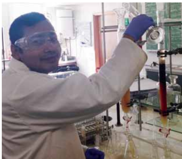
Dr Swarup (Postdoctoral Fellow) is doing column chromatography. Chromatography is a method of separation or purification. Silica components are separated according to their polarity.
