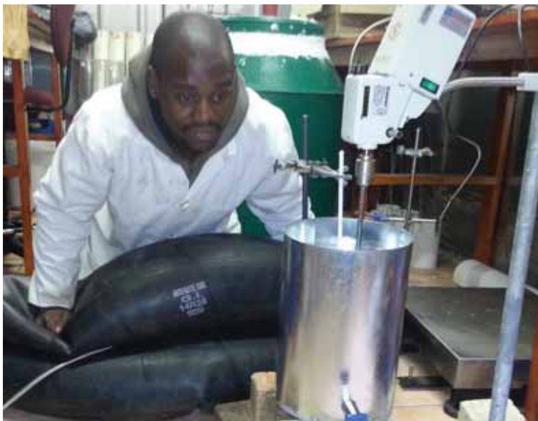
MSc candidate Mr Phindile Madikizela using biogas recovered from an anaerobic digester to pasteurise digested faecal sludge
